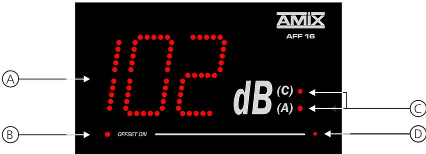
Acoustic pressure tendency display under A or C weighting. It can display error codes.
